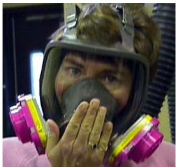
This test is very similar in principle to the negative pressure test. It is conducted by closing off or covering the exhalation valve and exhaling gently into the face-piece. The test is easy for respirators whose valve cover has single small port that can be closed by the palm or finger. If the face pieces remain slightly inflated and no outward leakage is detected, a proper fit is achieved.
