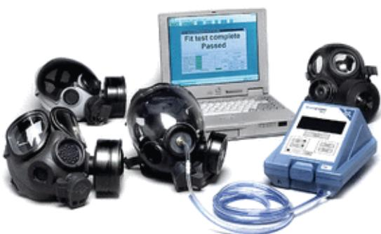
The airborne concentration of the substance is measured outside and inside the respirator while the wearer performs the required exercises. The
