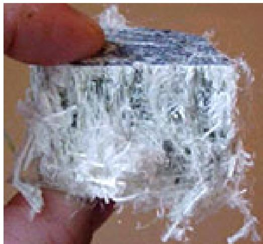
Picture of asbestos fibers
