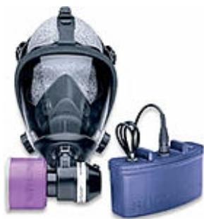
The advantage of using a powered air purifying respirator is that it maintains air at four CFM positive pressure within the face-piece, helmet or hood and at least six CFM to a loose fitting helmet or hood. This provides a higher degree of protection than half face and full - face air purifying respirators.
