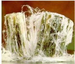
**Serpentine Asbestos (snake-like structure)**
