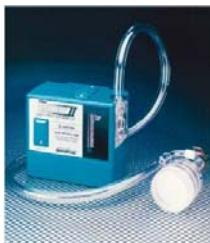
Battery powered, or personal sampling pumps, are small, lightweight pumps usually encased in a hard plastic shell. These pumps typically draw from one-half to 4 liters of air per minute through the filter and are ideal for indexing workers' exposure (or potential exposure, when wearing a respirator) to airborne asbestos fibers. Characteristically light weight, these pumps are easily worn on a worker's belt with little discomfort.
