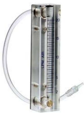
A rotameter is a device that measures the flow rates of sampling pumps in the field. It is considered a secondary standard of calibration because it is not as accurate and needs to be calibrated itself.
